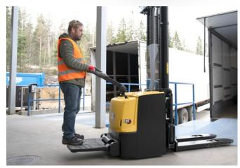
Models with a small fold-down platform are available at 1.0, 1.2, 1.4 and 1.6 tonne capacities to take the legwork out of longer distances.
