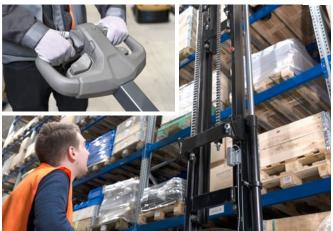
Smooth and precise control characteristics and a comfortable operating position, with a user-friendly tiller arm and excellent visibility through the mast, ensure a satisfying user experience. Height-adjustable castor wheels and high-strength masts help to maximise stability.
