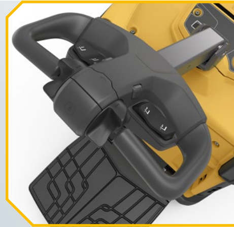
(Pictured right) The latest ergonomic tiller arm is designed for simple, comfortable use and minimal fatigue. Its large controls are easy to reach and to operate, even when wearing gloves.
