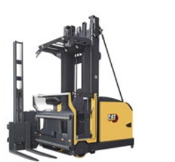
Man-Up Turret Trucks: 1.1 – 2.0 tonne capacity
