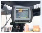
Rear-view camera (fitted as standard) combines with special mast, dashboard and overhead guard designs to give clear all-round views with little or no need for driver to lean or change position.
