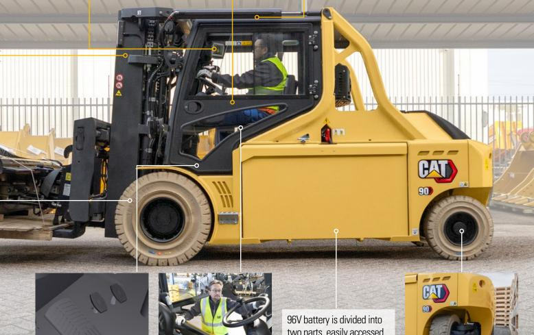
Separate forward and reverse pedals allow rapid changes of direction in busy operations and are accompanied by a large brake pedal for fast application with little effort. (Conventional pedal set is optional.)
