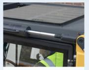
High-positioned mast tilt cylinders enhance stability, especially at greater heights, and increase residual capacity.
