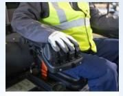
Fingertip hydraulic controls on a comfortable, adjustable armrest are standard on NH models and optional on N.
