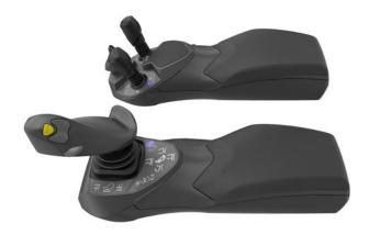
The dual joystick option separates functions such as clamp opening, to avoid accidental moves. It's especially useful for drivers who find fingertip levers too small to operate with gloves (or large hands).
